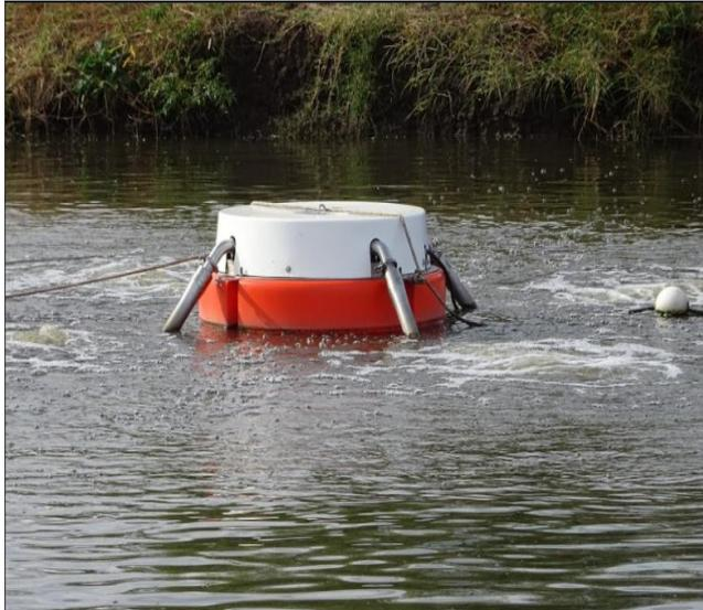
The aerator is positioned between the two raw water pumps (shown at left during installation) to deliver the maximum amount of aeration throughout the water body where raw water is harvested for treatment.
